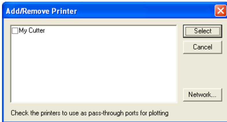
If you've installed a driver from your cutter's manufacturer or followed the steps above, it will appear in this window and you can place a checkmark next to it as shown above. Place a checkmark next to the cutter you want to use, and press **Select**.
