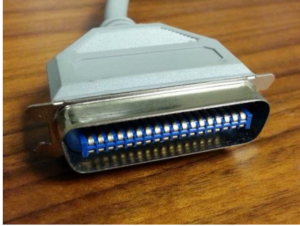
Centronics connector at the cutter end
