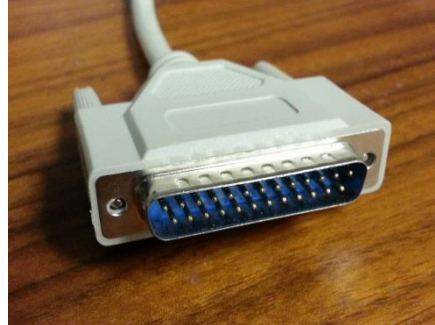
25-pin parallel connector at the computer end
